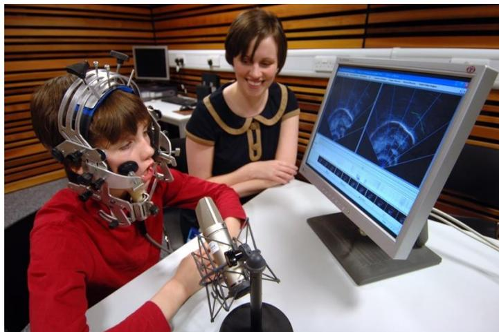
A picture of the ultrasound setup showing a child wearing the ultrasound headset and ultrasound images of the tongue on a computer screen
