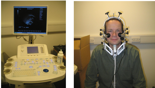
Fig. 3. Left: ultrasound machine used. Right: device to stabilise the head (to reduce motion wrt the ultrasound probe).
